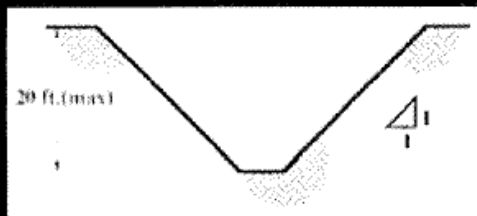
SIMPLE SLOPE TYPE B SOIL 20 ft. or less in depth maximum allowable slope of 1:1
